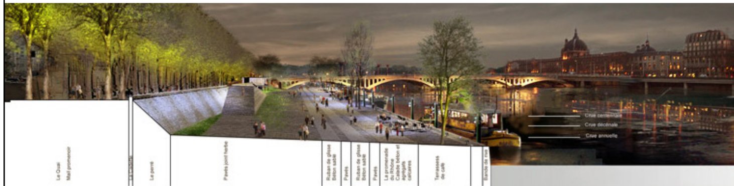
Section perspective cut from the upper main street level to the lower level along the riverbank.
